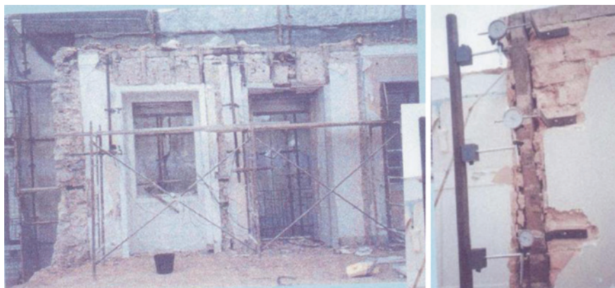
Fig. 9 In-situ tests to rupture [8]
