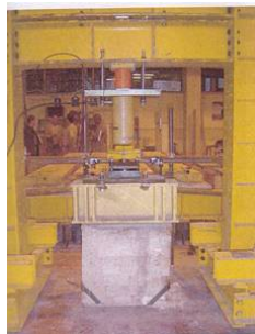
Figure 23 – Frame for monotonic compression test on masonry panel from Campo Pequeno Bullring (Branco and Correia, 2003).
