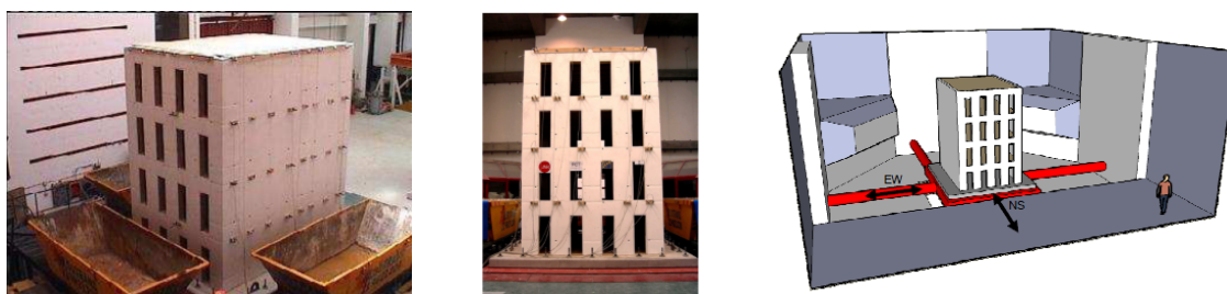
Figure 31 – Overview of the building prototype before test and test setup (Candeias, 2008).
