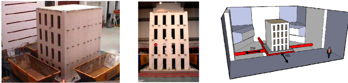
Figure 41 – Overview of the building prototype before test and test setup (Candeias, 2008).
